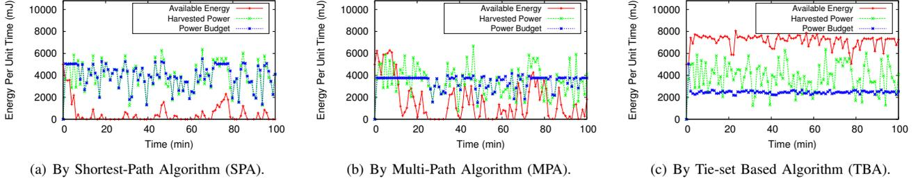
Fig. 4. The simulated behavior of available energy  $a_i(t)$ , harvested power  $g_i(t)$ , and power budget  $pF_i(t)$  from  $t = 0$  to 100 (min) at a node  $v_i \in V$ .
