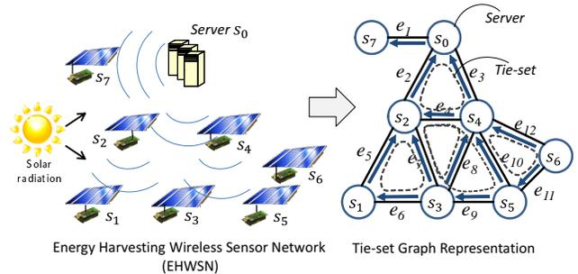
Fig. 1. Graph representation of an EHWSN and a routing example based on tie-sets.
